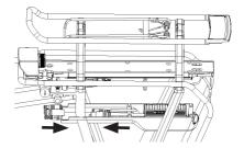
Position the controller holder under the battery rail, and with 6 X ST3\*19 screws tighten the controller holder to the battery rail. Tightening torque requirement: 3 Nm.
