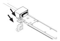
Place the battery rail in position on the luggage carrier, and with 3 X M5\*25 secure the battery rail to the luggage carrier by tightening the screws. Tightening torque requirement: 3 Nm.
